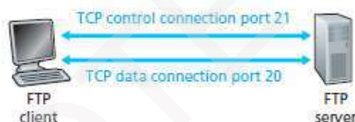
Figure 1.10: Control and data-connections
